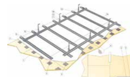
M643 Installation diagram (M643) for Ecophon Fade Duo Smooth suspended grid, glued to substrate
