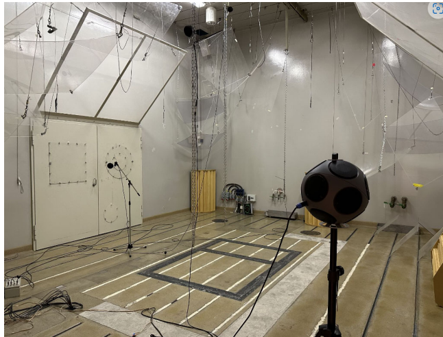
Picture 3 and 4: Loudspeaker and Microphones for L_{W0} measurements All in all 2 loudspeaker positions and 8 microphone positions for each one of these.
