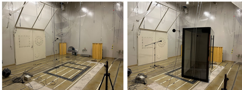
Measurement of T_0 and T_1 according to ISO354.
