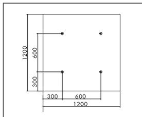
Suspension with absorber anchor, format 1200 x 1200
