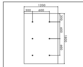
Suspension with absorber anchor, format 1800 x 1200
