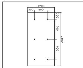
Suspension with absorber anchor, format 2400 x 1200
